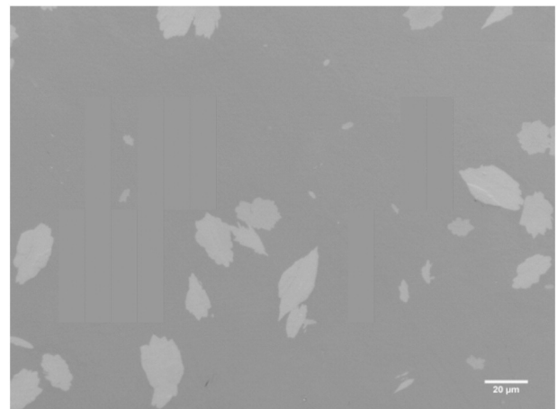
Fig. 2. Optical micrograph of a lithium disilicate glass-ceramic obtained by annealing glassy lithium disilicate for 90 h at 500^\circ\text{C} .
