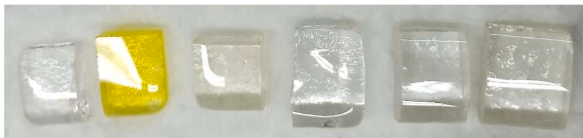
Photographs of the prepared samples, left to right, Eu10, CdS10, Eu10_CdS10, Eu10_CdS20, Eu10_CdS30 and Eu10_CdS50
