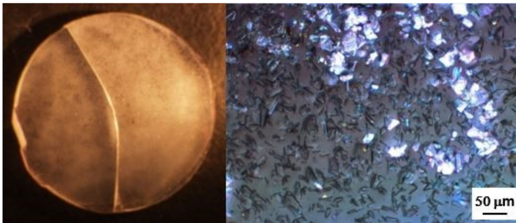
FIGURE 8 B3B fractured piece from the B2 sample treated at T_g for 1 h. Top (left) and cross-sectional (right) views of the sample showing a large number of microcracks
