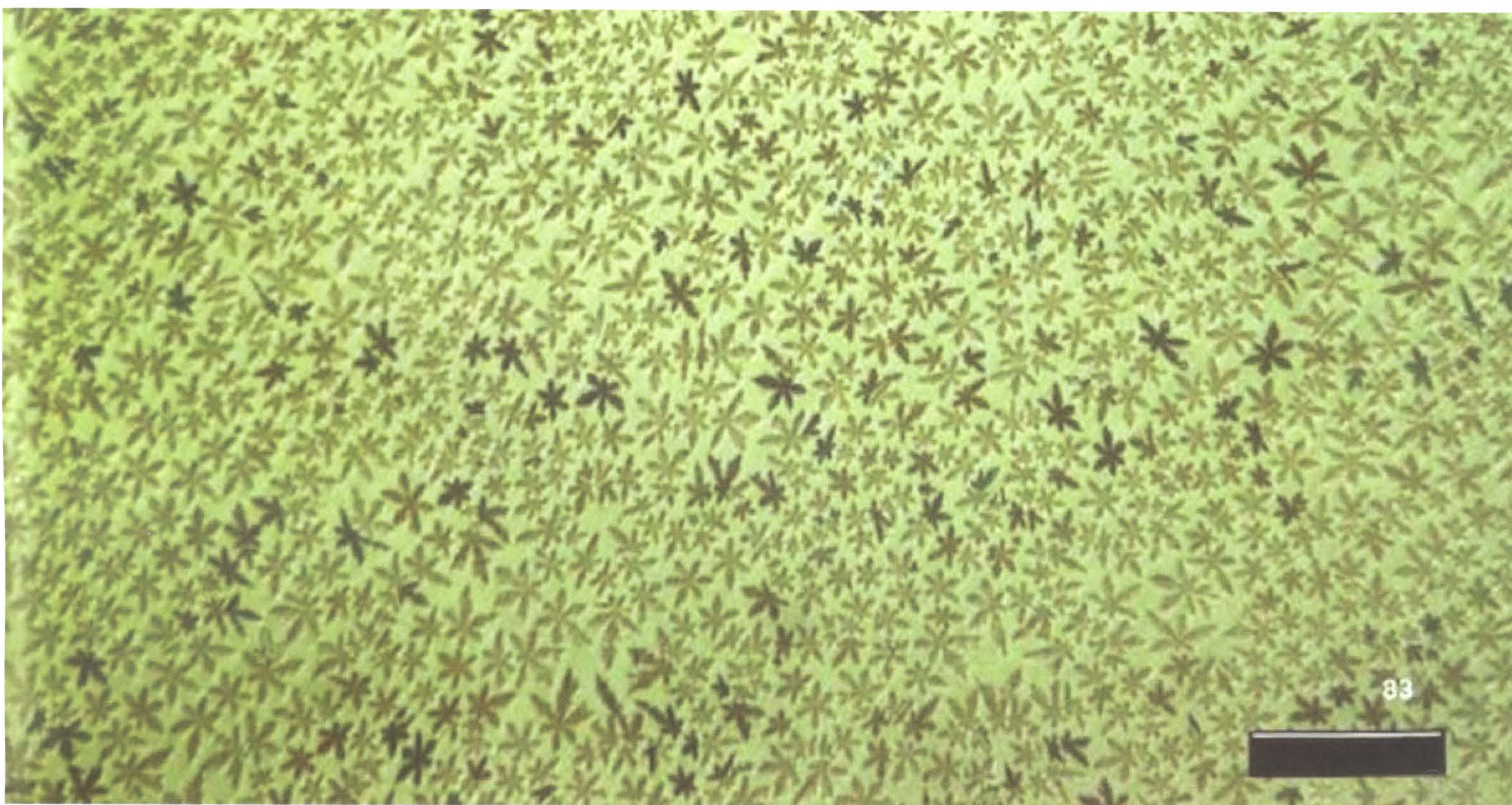
Optical micrograph showing a plethora of lithium metasilicate crystals embedded in the residual matrix of a rare (nucleant-free) glass-ceramic. The bar indicates 100 micrometers.
