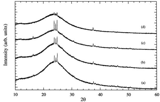
Fig. 1. XRD traces of heat-treated  $\text{LS}_2$  glass (a)  $454^\circ\text{C}$  for 360 h, (b)  $477^\circ\text{C}$  for 120 h, (c)  $477^\circ\text{C}$  for 168 h, and (d)  $500^\circ\text{C}$  for 24 h.
