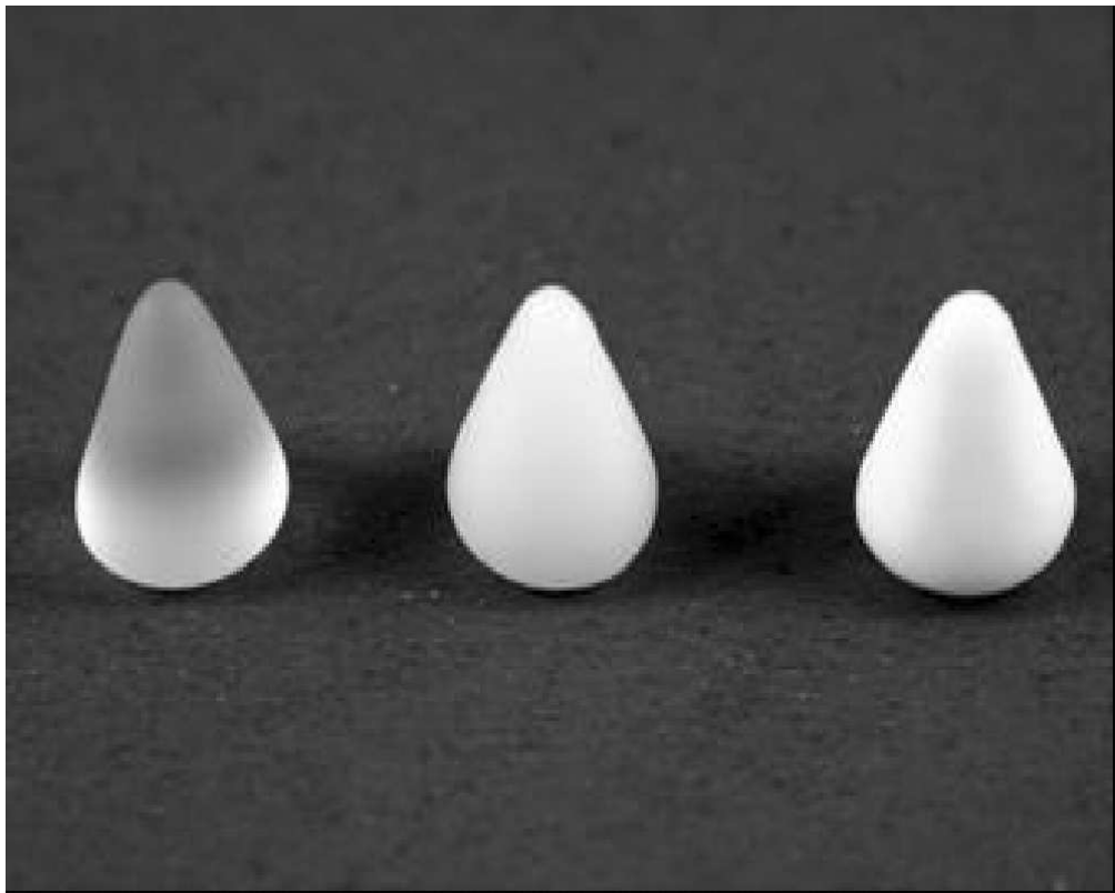
Fig. 1.Implants used in the study. A) Bioactive glass (Bioglass); B) Single-phase bioactive glass ceramic (Biosilicate 1P); C) Double-phase bioactive glass ceramic (Biosilicate 2P). 84x67mm (300 x 300 DPI)
